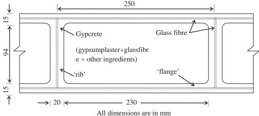
Fig. 1. Enlarged view of a typical cell of GFRG panel
