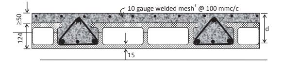
Fig. 3.Typical cross-section of panel with micro beams
